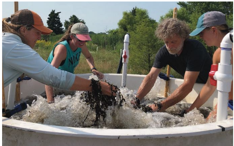
FIGURE 5 Volunteers from Anne Arundel Community College, Shore Rivers and Submerged Aquatic Vegetation Watchers use the turbulator to separate seed from stems of Potamogeton perfoliatus (Redhead grass).
